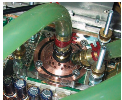
Figure 8b. Angular Introduction of Coolant with Central Return of the Heated Fluid [1].
